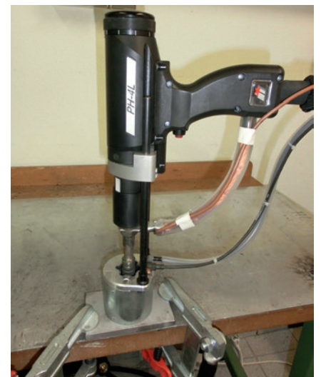
Fig. 4 • SRM welding gun for M16 studs – the connection of the magnetic field shielding gas fixture to the support feet of welding guns and welding heads is also easily possible with stationary handling.
