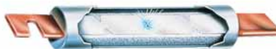
Figure 2. Under sustained overload, a section of the link melts and an arc is established.
