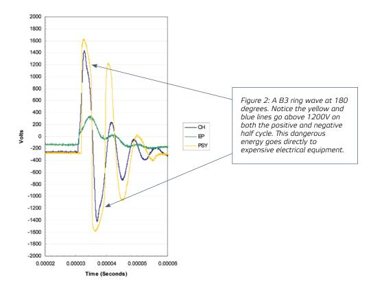
"Again, the important number to analyze here is the let through voltage. CH let through more than three times as much as EP, while Psy let through more than four times as much voltage as EP," said Joseph. "Protecting equipment from these two ring waves is critical to the efficient operation of the loads."
