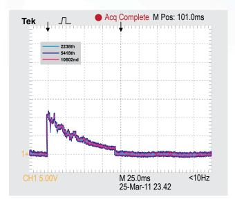
Figure 3 clearly shows EP's waveform correction technology maintains its attenuation levels after more than 10,000 surges. Typical MOV based technology degrades with each surge and does not protect from A1 or B3 ring waves.
