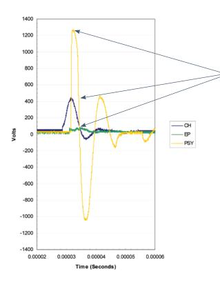
Figure 1: An A1 ring wave at 180 degrees. The green line represents EP. The blue line represents Cutler Hammer and the yellow line represents Psytronics. The higher the line goes the more danger there is to equipment.
