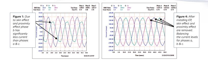
Current should flow through the center of the conductor, however noise causes the flow of current to be pushed to the circumference of the wire. This is known as skin effect.
