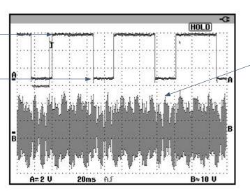
The negative half cycle is almost indistinguishable from the positive half cycle. The noise on the waveform completely corrupted the communication channel.
