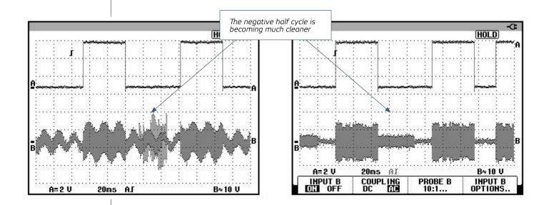
While these readings clearly show a strengthening of the signal, the negative half cycle is still polluted with high frequency noise.
