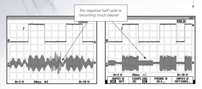
Figure 2 shows the high frequency content after installing additional EP filters. The positive and negative half cycles show significant noise reduction compared to Figure1. However the signal is still polluted with enough high frequency noise to interfere with the communication channel. The negative half cycle is beginning to smoothen but more filtration is still necessary.
