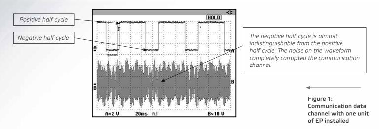
Figure 1 shows the data sent over the communication channel. Channel A is reference communication channel while the channel B is the actual data. The actual data is extremely corrupted and unusable.
